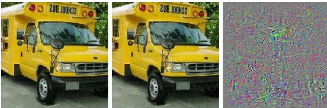
Left: An image that a neural network correctly classifies as a school bus. Middle: A very similar image that the neural network does not classify as a school bus. Right: A magnified view of the difference between the left and middle images. (Szegedy et al., 2013)
